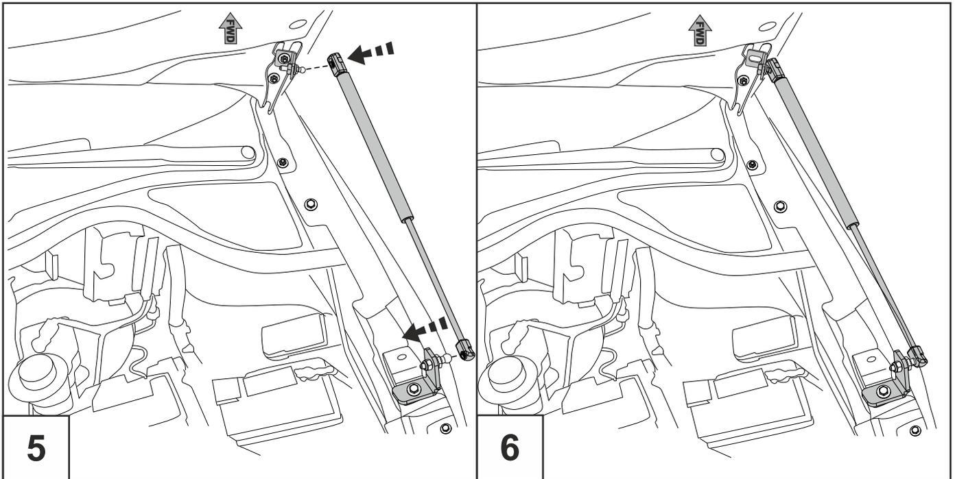
**GB** Holding the hood, remove a regular stop in the transport position and install the gazLift.
