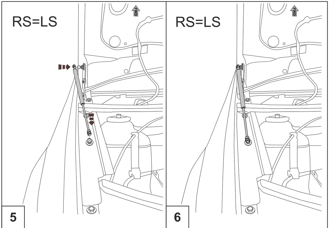
**GB** Holding the hood, remove a regular stop in the transport position and install the gazLift.
